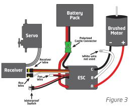
ESC) is not used. After calibration (See "How to Calibrate the ESC", page 10), you may need to swap the two motor wires to get the wheels to spin in the right direction.
